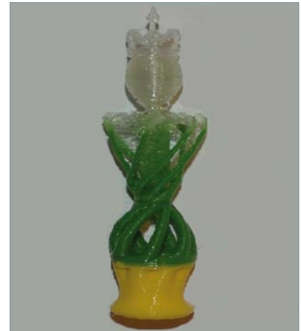
Figure 14. Model produced with three different filaments.
