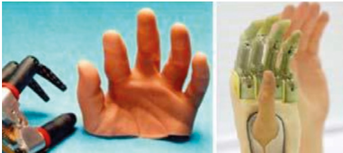
Figure 5. First ProDIGITS design vs. later design (Castellanos, et al., 2011).
