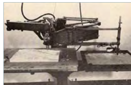
Figura 2. Pantógrafo (Institute of Cartography and Geoinformation, ETH Zurich, 2014).
